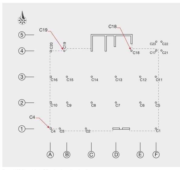
Figure 62(a): Plan of the building showing column locations
