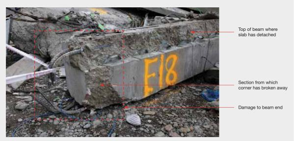
Figure 63(a): Edge beam from line 4 between lines A and B (source: Robert Heywood)
