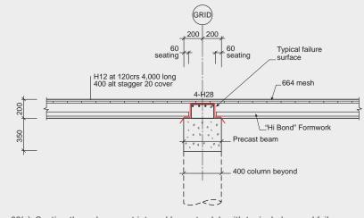
Figure 63(c): Section through precast internal beam to slab with typical observed failure surface indicated in red
